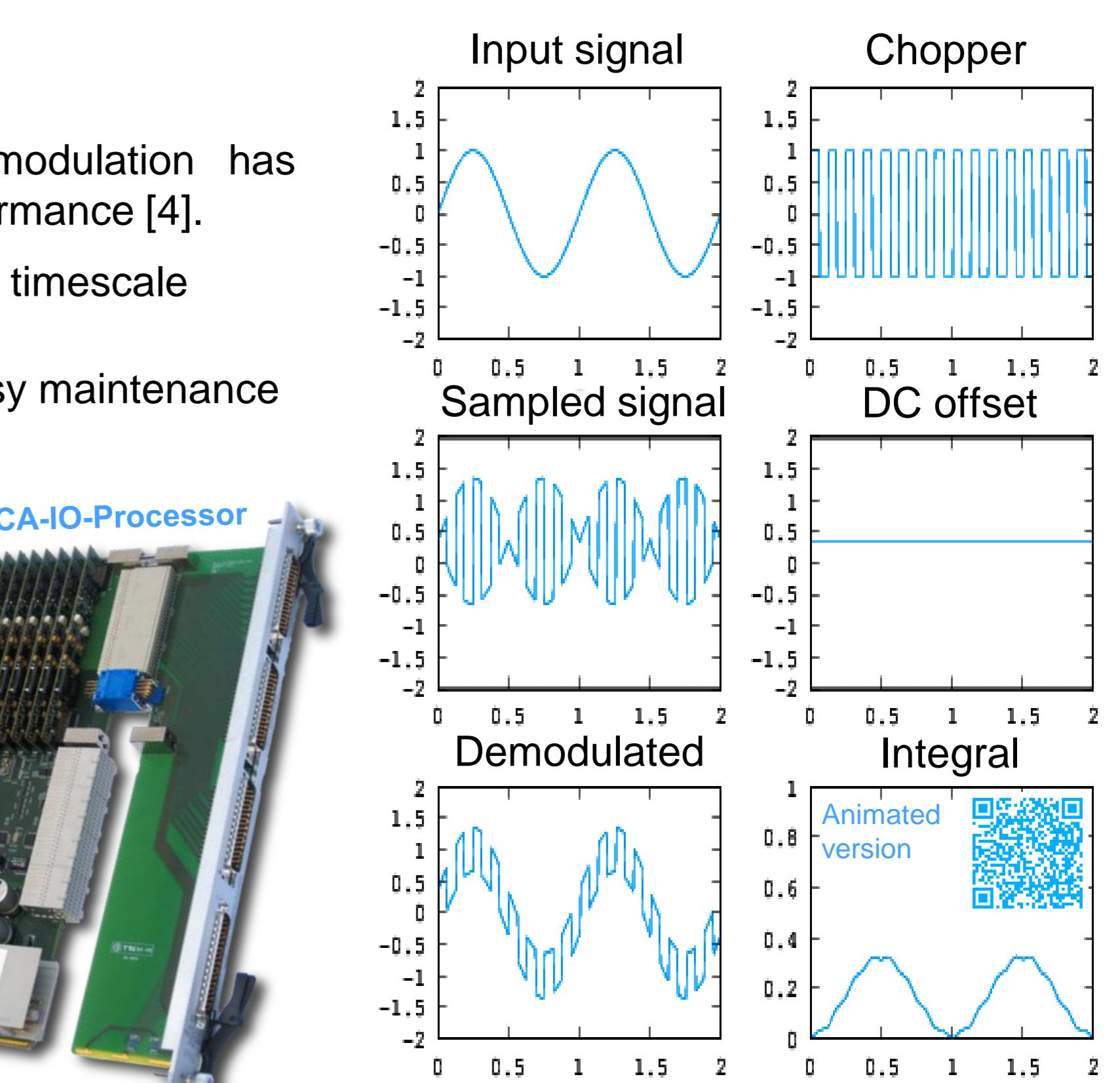
Phase modulation removes drift-inducing electronics offsets without affecting the integral
