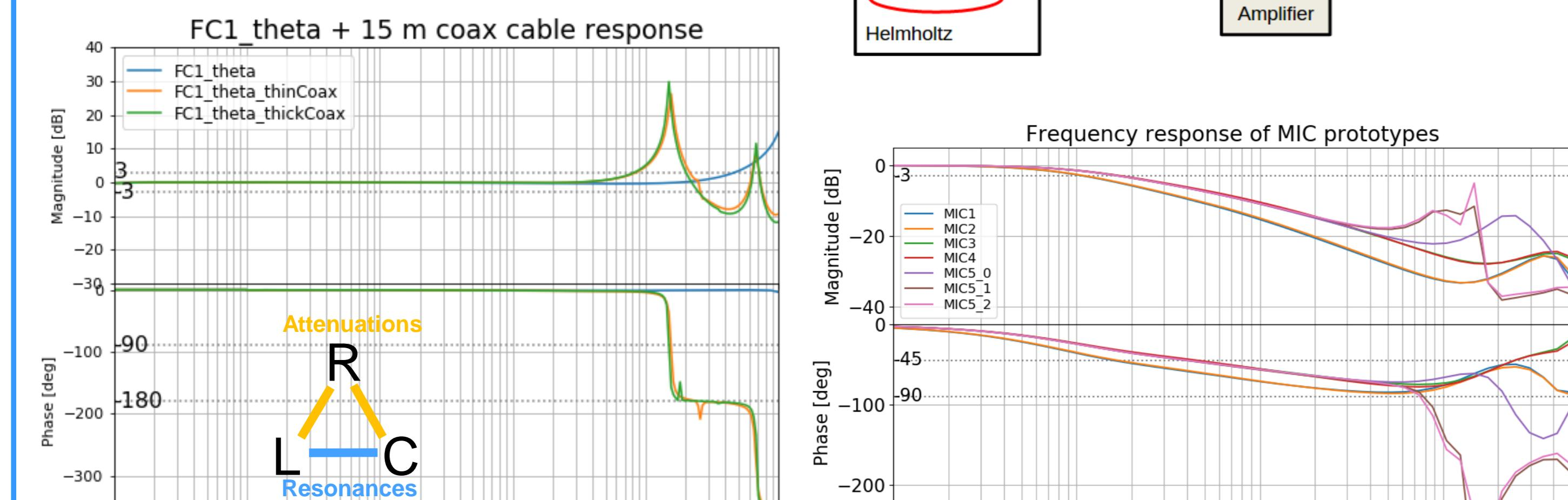
The knowledge of the frequency response of the full signal path allows its compensation using DSP and if not possible, the establishment of operating ranges and uncertainties
