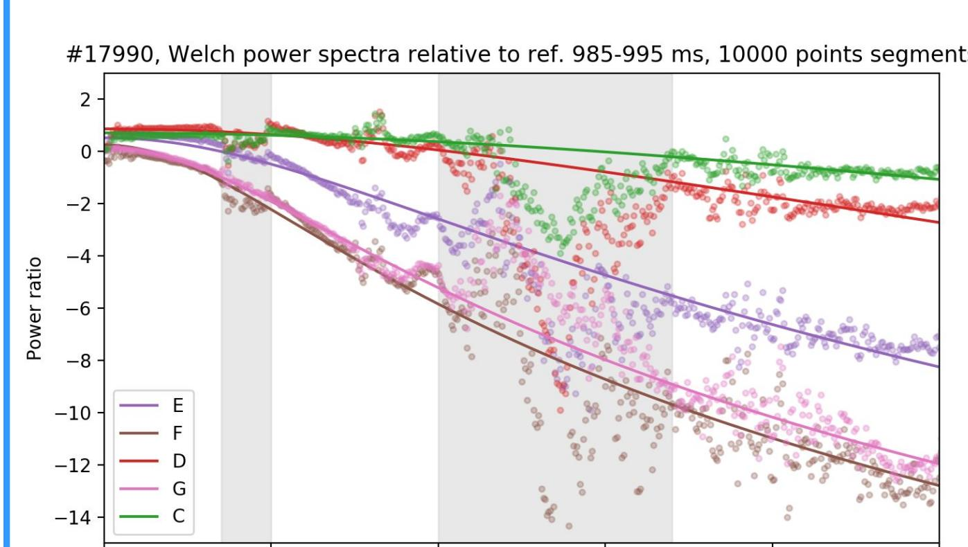
Frequency response comparable to first order filter: only shielding effect
