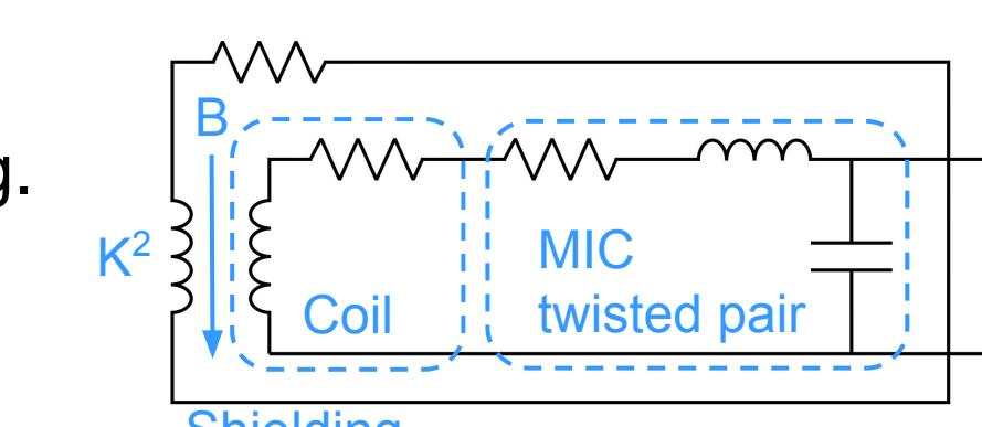
With the fitting results the model can be used to predict the behaviour of prototype coils and use the geometry of the coil and impedance of external circuit to extend the passband
