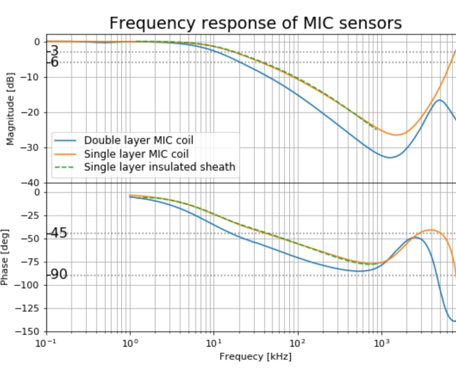
MIC Mirnov coils show bandwidths on the 10-20 kHz range
