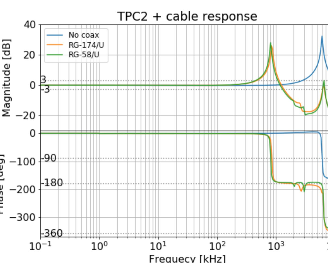
Using the measured parameters, extrapolations can be made for different lengths of cable and input impedances of DAS. Low probe and DAS capacitances ensure plasma oscillations up to 600 kHz can be accurately measured.
