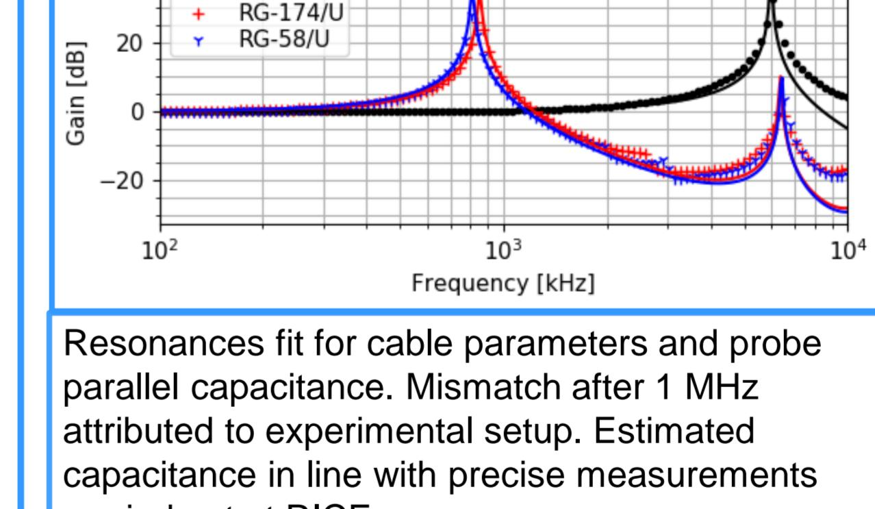
Resonances fit for cable parameters and probe parallel capacitance. Mismatch after 1 MHz attributed to experimental setup. Estimated capacitance in line with precise measurements carried out at RICE.
